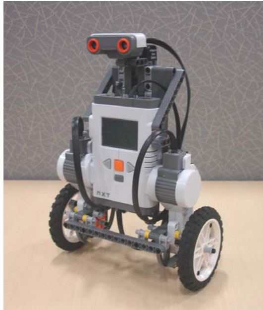
Figure 1.2: Yorihiya Yamamoto's balancing robot
